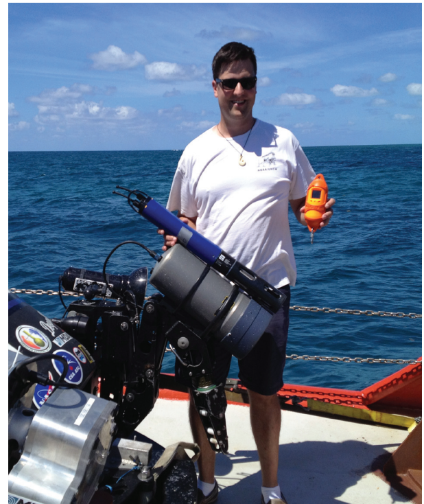
Art Trembanis displays the orange CastAway CTD and blue EXO2 multiparameter sonde that added sophisticated data-gathering capabilities to the NEEMO 16 mission in June 2012 and proved the remarkable versatility and convenience of both instruments.
